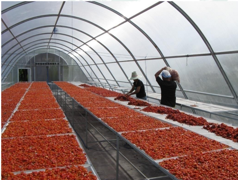
Drying in a parabolic greenhouse solar dryer
