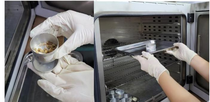
Place the sample in hot air oven at 105°C for 24 h
