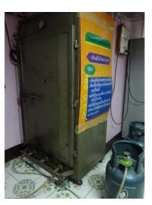
Drying using a tray dryer
