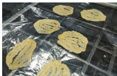
Drying in Solar Dryer until water activity < 0.6
